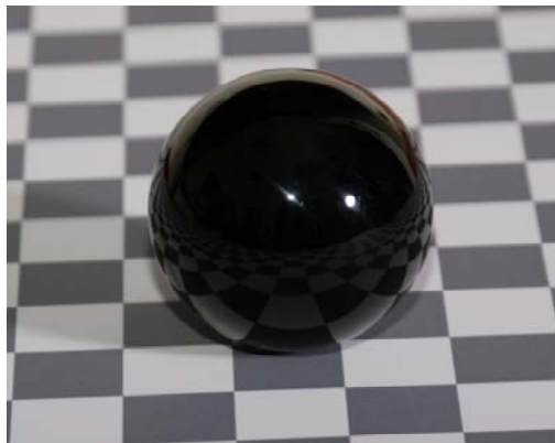
Figure 5.3.4-1. There are two specular highlights on the black sphere, created by two white light sources which are in front and to the right of the sphere.
