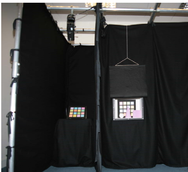
Figure 8.1.1-1. The lighting booth showing the palette (left) and 3D scene (right) compartment. The light source for the palette compartment is visible on the top left.
