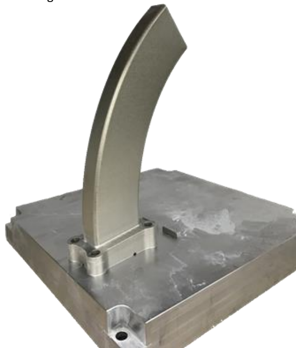
Figure 8 Build plate of the EOS M290 with manufactured component on it.
