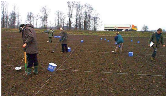
Figure 22: Systematic metal detector survey of an area that has been divided into grid cells.
