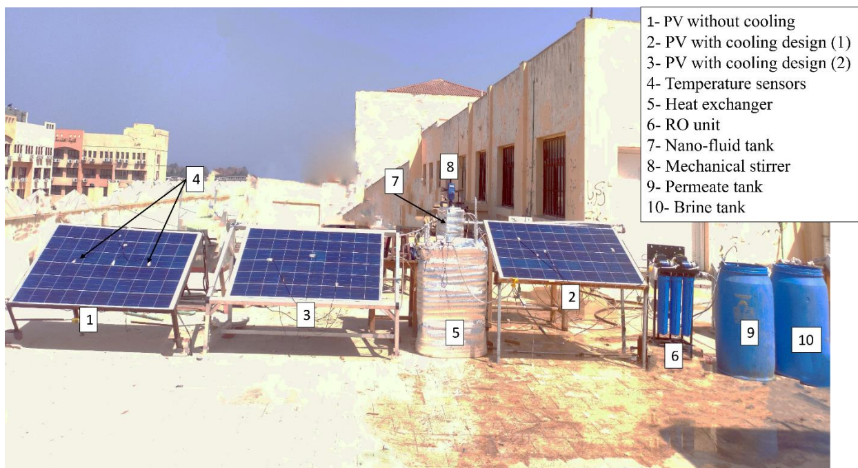
Fig. 1. Experimental test rig of the PV-RO integrated with two cooling/preheating design systems.
