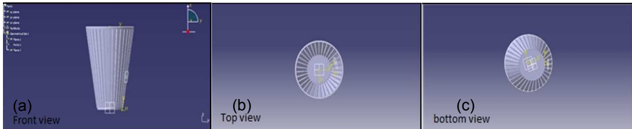
Fig. 1 Geometrical model of perforated rotating bucket in 3D, (a) front view, (b) top view,(c) bottom view
