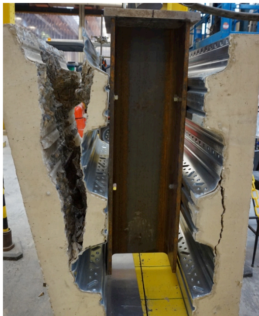
Figure 5: Failure mode of the push test with 100mm bolted connectors
