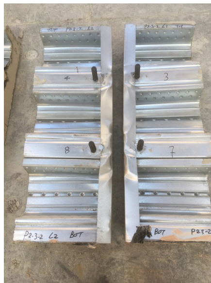
Figure 11: Push test specimen with full depth edge trim
