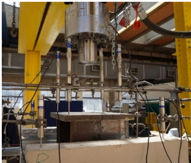
Figure 2: Positions of LVDTs
