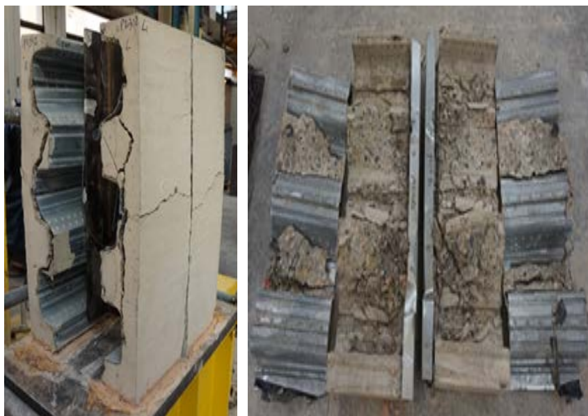
Figure 15: Specimen after the push test
