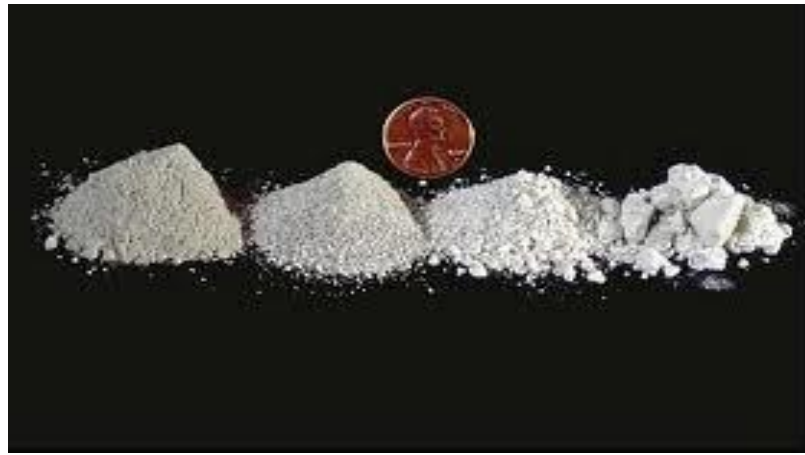
Figure 1.2.1: Tephra particle sizes ranging from ash (left hand two piles) to Lapilli (right hand two piles). Taken from http://volcanoes.usgs.gov/about/pglossary/tephra.php .
