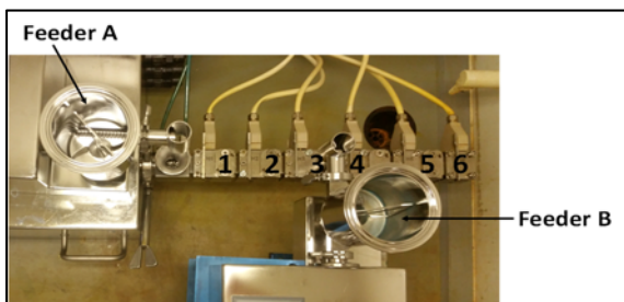
Figure 2: Twin screw extruder, consisting of six heating sections with two attached volumetric feeders (A and B).
