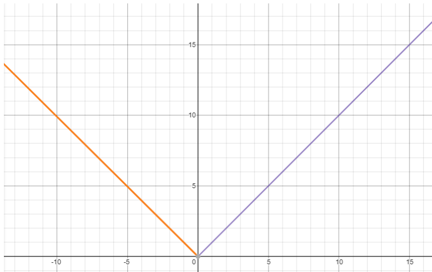
Figure 3. The modified Quantum ReLU (m-QReLU) activation function.
