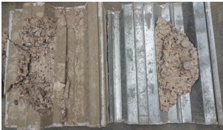
Figure 7. Concrete pull-out failure mode observed from test specimen M7
