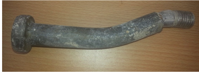
Figure 14. Deformed shape of shear connector in test specimen M2
