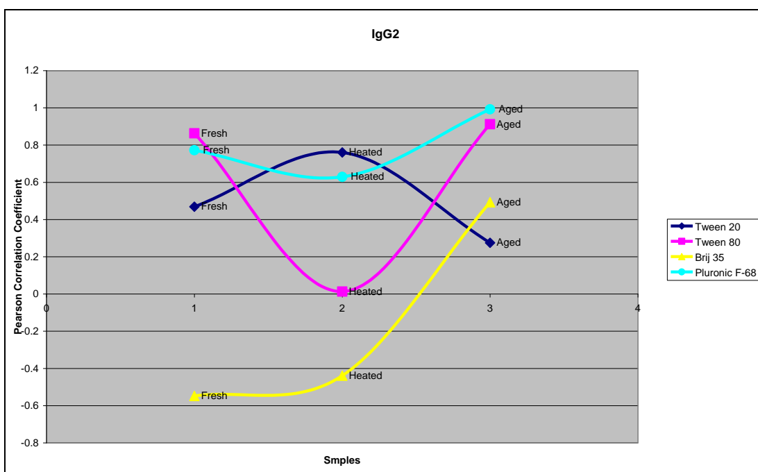
Figure 6.10. The Pearson Correlation Coefficient between HSDSC unfolding temperature T_{m1} and main peak diameter (nm) measured by DLS for: (1) fresh, (2) heated and (3) aged IgG2 with Tween 20, Tween 80, Brij 35 and Pluronic F-68 surfactants.
