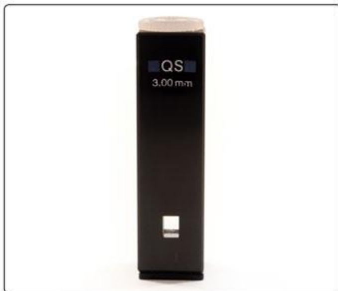
Figure 2.3. Low volume quartz batch cuvette for size and molecular weight measurements for use with the Zetasizer Nano series (The Nanobiotechnology Centre, 2009).
