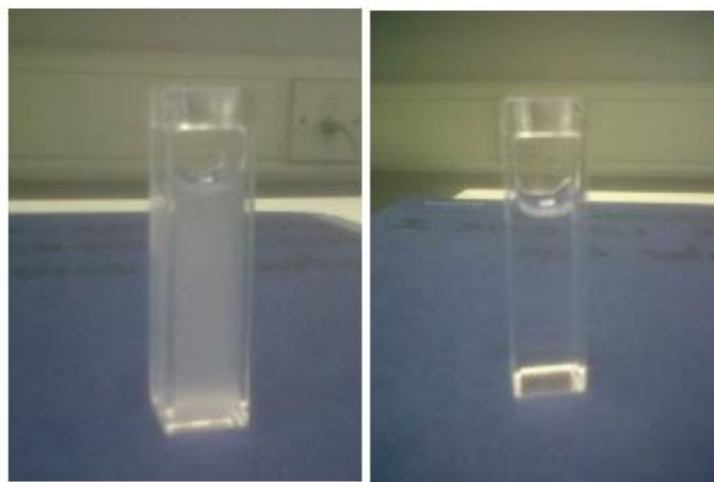
Fig. S23 – Turbidity (cloudiness) of PAA + PAM at pH 2 (left) and 7 (right) at 0.2 mg ml -1
