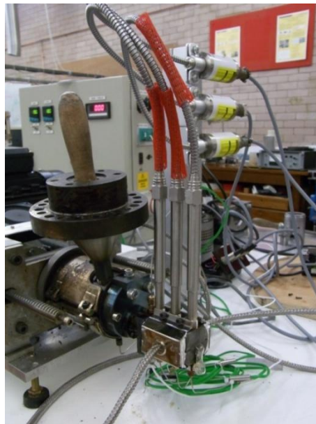
Figure 3.10: Slit die with pressure transducers
