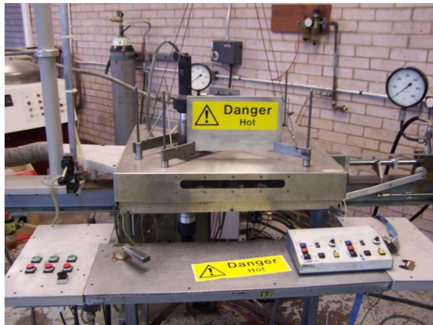
Figure 3.13: Setup of the biaxial stretcher
