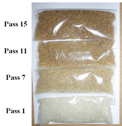
Figure 3.17: The different colour complexity of each run after extrusion in the APV
