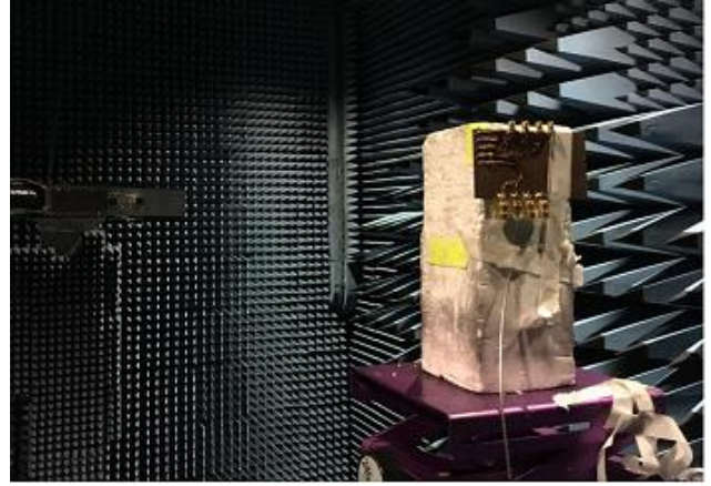
Fig. 17. Measurement setup for the radiation patterns.
