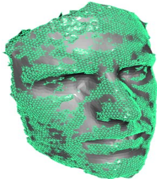
Figure 9. Comparison of scan facial data (shown in mesh format) with the reconstructed face (shown as shaded)
