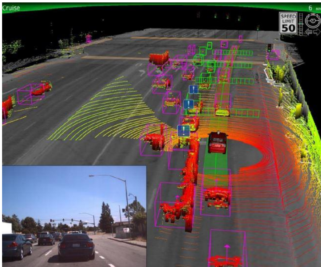
Figure 2-7: How Autonomous vehicles see the road (Md, 2015)
