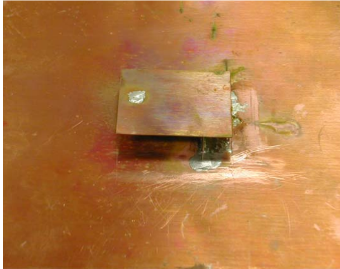
Figure 6.35 Photograph of the fabricated harmonic rejection antenna with a shorting wall.
