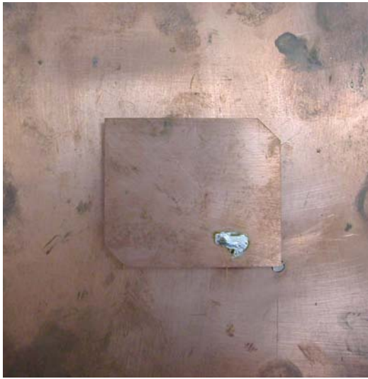
Figure 6.25 Photograph of a fabricated prototype antenna with two cutoffs at corner for CP.
