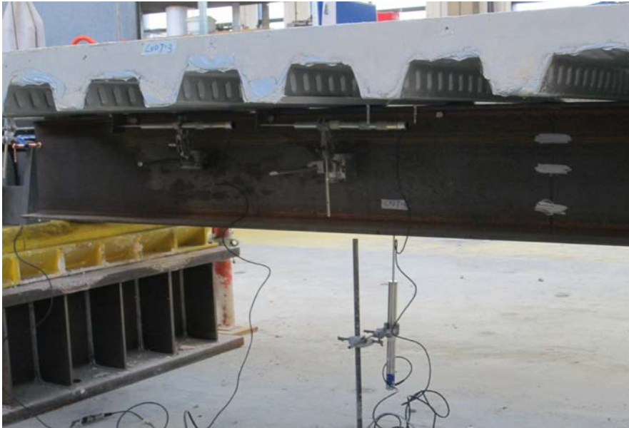
Fig. 13. LVDTs at the 2 nd and 4 th shear connector's position
