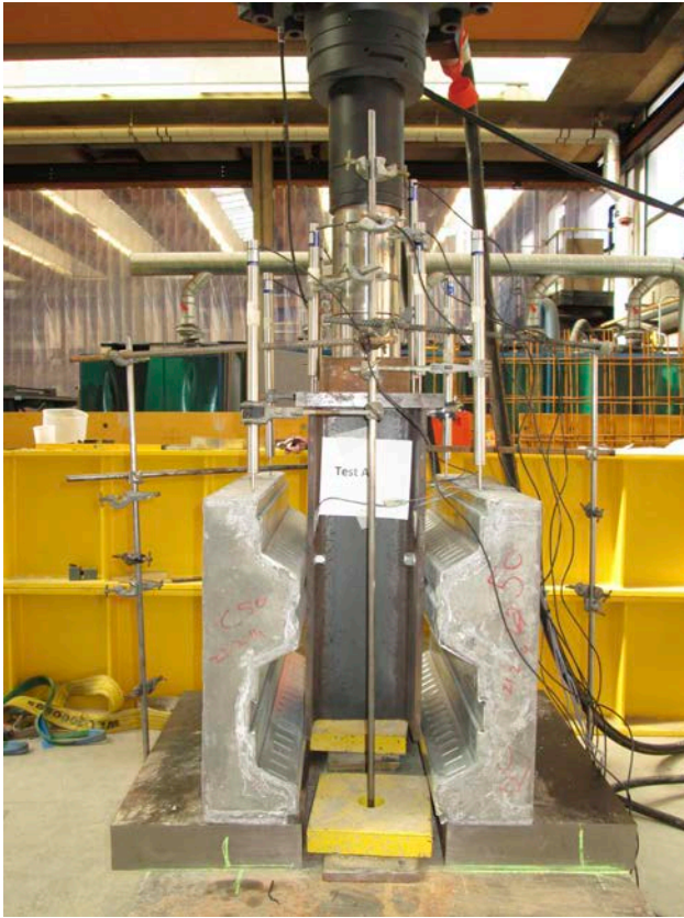
Fig. 2. Push test set up and test arrangement
