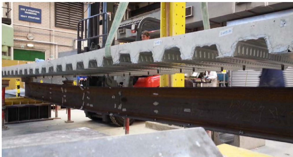
Fig. 16. Demountability of the composite beam
