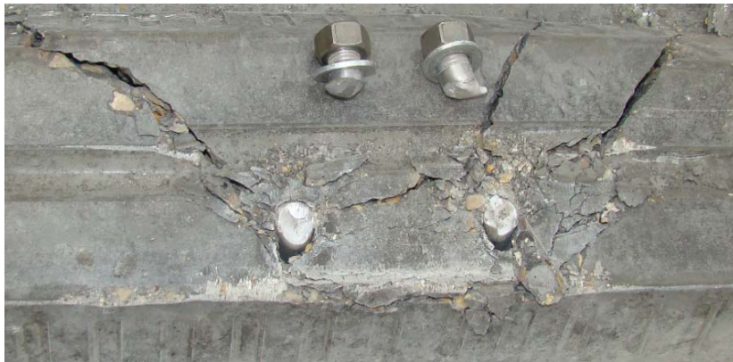
Fig. 4 Fracture of the shear connectors
