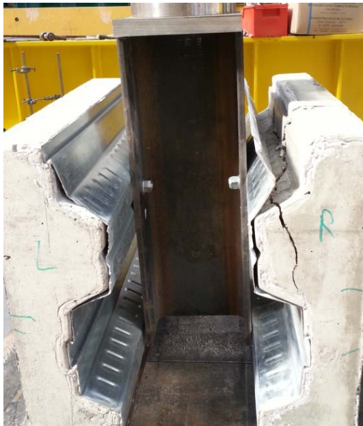
Fig 5. Rib shear failure to the concrete slab
