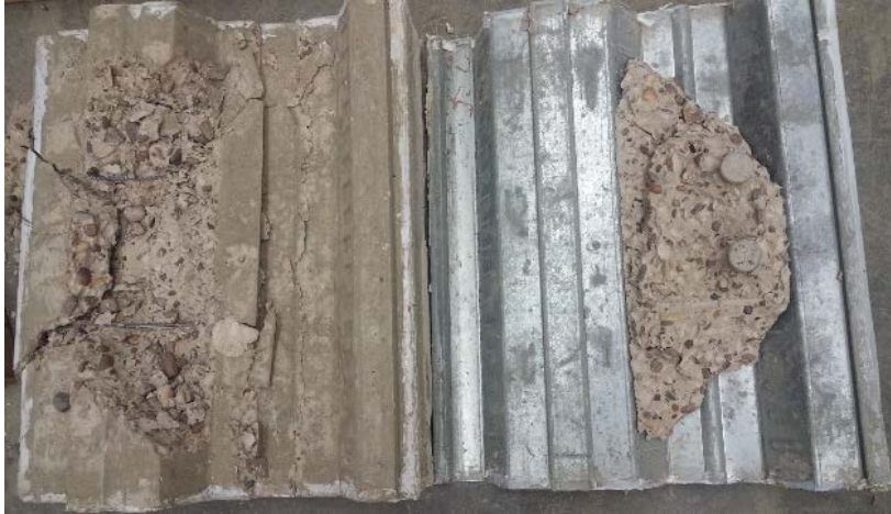
Fig. 3. Concrete cone failure observed from test specimen M7
