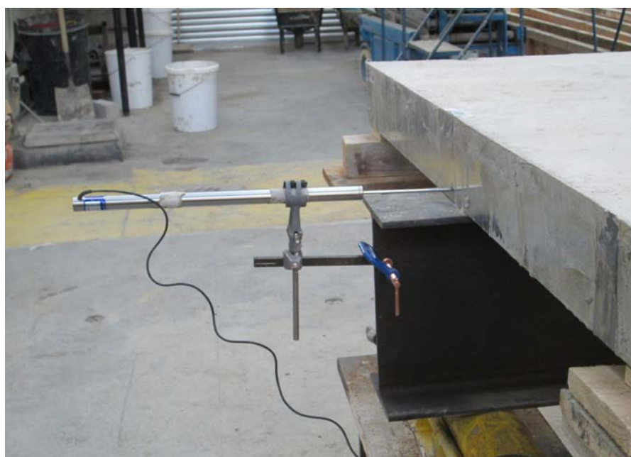
Fig. 12. LVDT for the end slip
