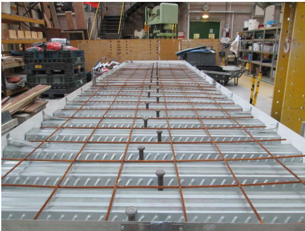
Fig. 9. Set up before casting of the composite beam
