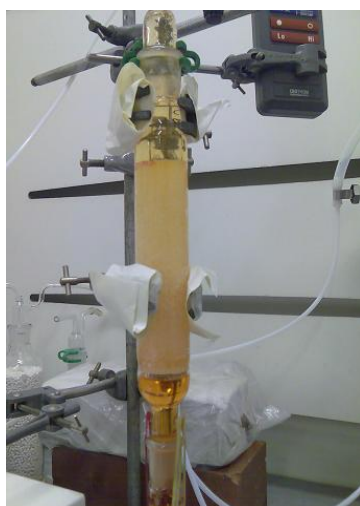
Figure 3: Dye ozonation experiment with silica gel
