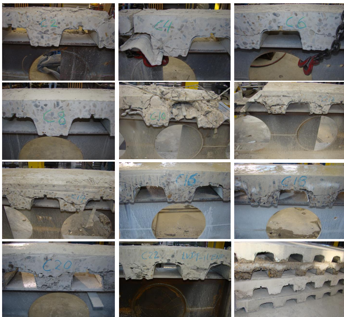
Figure 21 Failure mode of concrete slab
