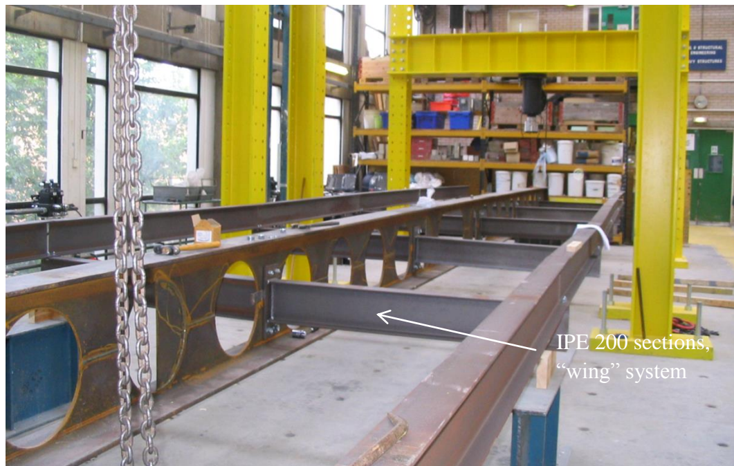
Figure 3 “Wing” system used to support wet concrete slab weight
