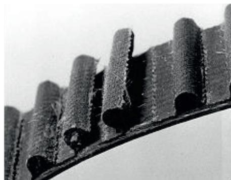
Fig. 1 – Timing belt failure mechanism; tooth root cracking
