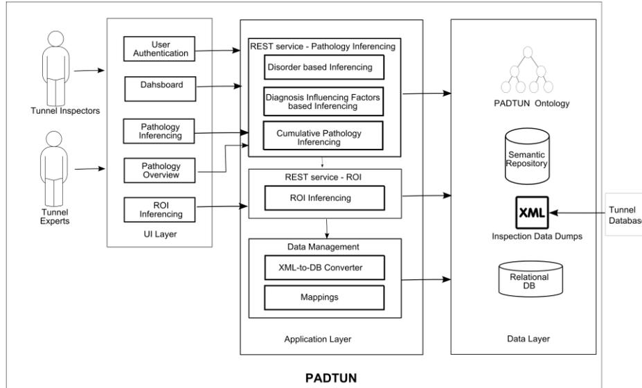
Fig. 1. PADTUN system architecture
