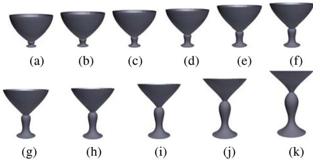
Figure 3. Sequence showing how the source surface  $S_s$  has been morphed into the target one  $S_t$  by using a gradual change in the boundary conditions and finding each of the intermediate surfaces via the proposed PDE method.
