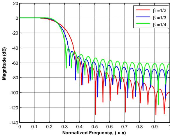
Figure 1: Side-lobes of root-raised cosine filter function
