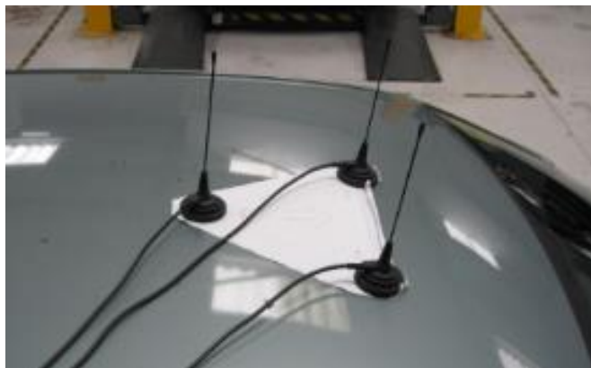
Fig.1. Measurement antenna setup (receiver)
