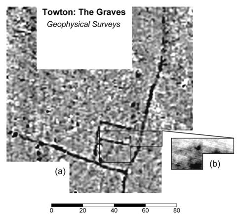
Figure 3: Geophysical survey data over a level piece of ground showing a premedieval field system incorporating a small enclosure and modern ploughing. (a) Fluxgate gradiometer survey (FM36) at  $1m \times 1m$  resolution, range  $-1.5 \dots +1.5nT$  (white to black). (b) Earth resistance survey (RM15, 0.5m twin probe) at  $0.5m \times 0.5m$  resolution range  $33 \dots 42\Omega$  (white to black).
