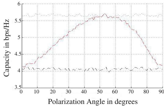
Figure 2: The channel capacity of  $2 \times 2$  MIMO system as oriented in Figure 1 as a function of the polarization angle. ('...': upper limit of  $2 \times 2$  MIMO fading channel, '-.-.-': upper limit of  $2 \times 1$  MIMO fading channel, Capacity using Eq. 1: red line, Capacity using Eq. 15: blue dots).
