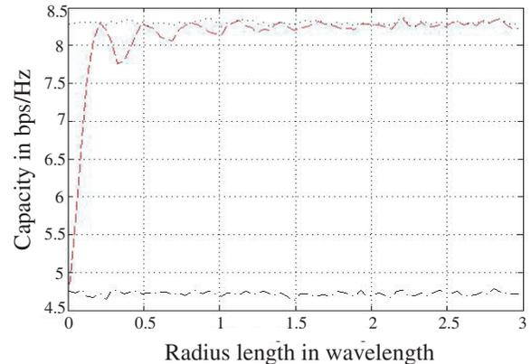
Figure 7: The channel capacity of  $3 \times 3$  MIMO system as oriented on a ring (the antennas are located at  $0, 120$  and  $-120$  azimuth angles) as a function of the radius distance in wavelength (c). ('...': upper limit of  $3 \times 3$  MIMO fading channel, '-.-.-': upper limit of  $3 \times 1$  MIMO fading channel, red line, Capacity using Eq. 2: blue dots).
