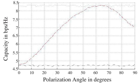
Figure 3: The channel capacity of  $3 \times 3$  MIMO system as oriented in Figure 1 as a function of the polarization angle. ('...': upper limit of  $3 \times 3$  MIMO fading channel, '-.-.-': upper limit of  $3 \times 1$  MIMO fading channel, Capacity using Eq. 1: red line, Capacity using Eq. 2: blue dots).
