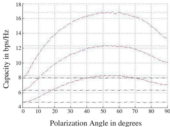
Figure 6: The channel capacity of  $3 \times 3$  MIMO system as oriented in Figure 1 as a function of the polarization angle for different SNR starting from 10 dB, 15 dB and 20 dBs. ('...': upper limit of  $3 \times 3$  MIMO fading channel, '-.-.-': upper limit of  $3 \times 1$  MIMO fading channel, Capacity using Eq. 1: red line, Capacity using Eq. 2: blue dots). The elevation angle is varied uniformly over 180 degrees at the horizontal plane.
