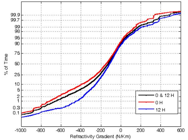
Fig. 3. Cumulative distributions of refractivity gradient at 100 m
