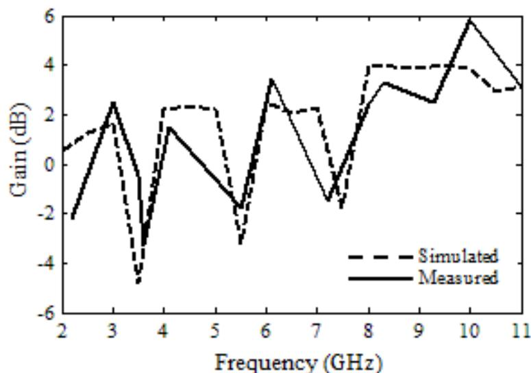
Fig. 13 Simulated and measured realized gain versus frequency
