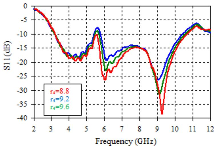
Fig. 5 Reflection coefficient for different values of r4
