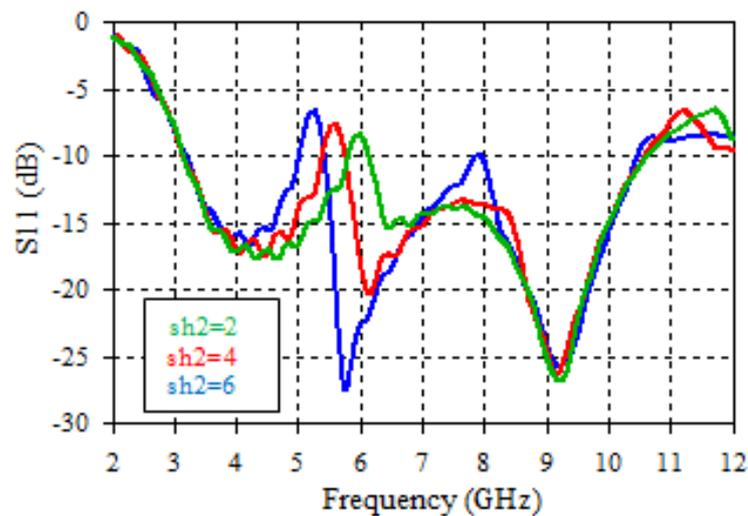
Fig. 4 Reflection coefficient for different values of sh2
