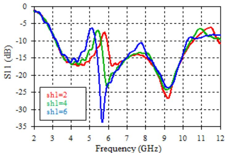
Fig. 3 Reflection coefficients for different values of  $sh_1$
