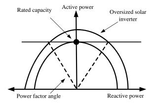
Fig.2. Capability curve of PV inverter
