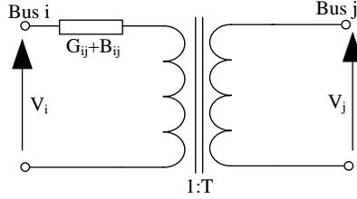
Fig.3. Model of a generic branch
