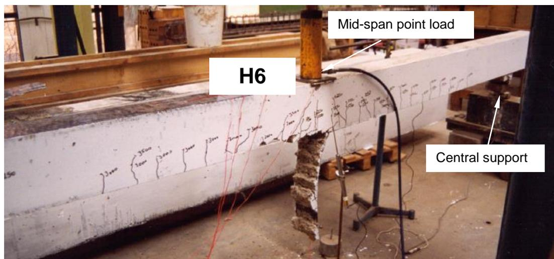
Figure 4 Peeling failure of the concrete cover initiated from the soffit CFRP sheet end near the central support (beam H6)
