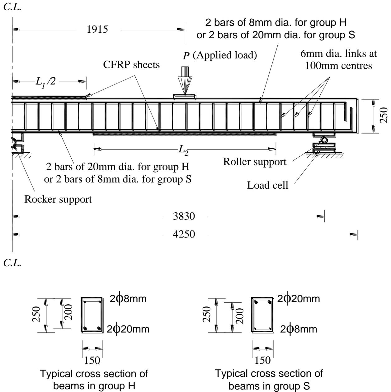
Figure 1 Geometrical dimensions, reinforcement and test rig of test specimens
