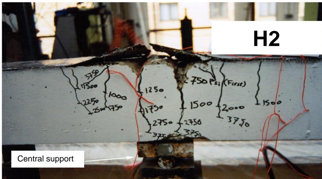
Figure 3 Tensile rupture of the CFRP sheets (beam H2)
