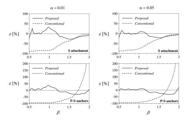
Comparison between proposed (solid lines) and conventional (dashed lines) CQC rules for the S attachment (top) and the P-S anchors (bottom); tuning parameter in the range  $0.5 \le \beta \le 2.0$ ; mass ratios  $\alpha = 0.01$  (left) and 0.05 (right).
