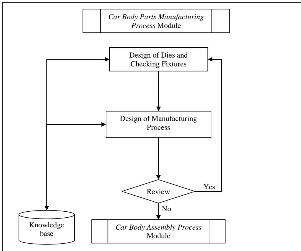
Figure 7.4: Flowchart of *Car Body Parts Manufacturing Process* module
