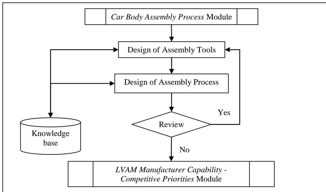
Figure 7.5: Flowchart of *Car Body Assembly Process* module
