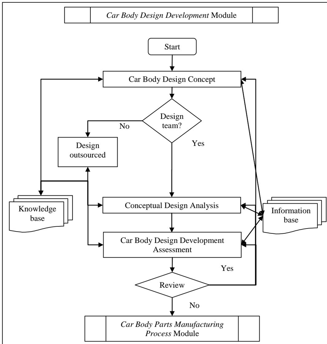
Figure 7.3: Flowchart of *Car Body Design Development* module
