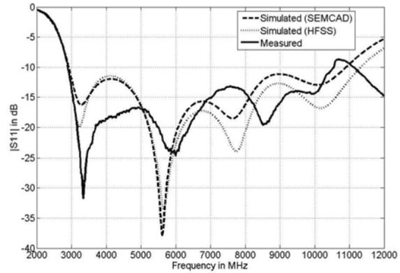
Figure 2 Measured and simulated reflection coefficients  $|S_{11}|$
