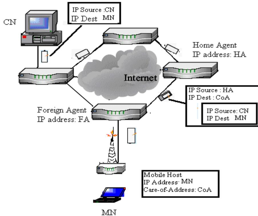
**Figure 2.1: Mobile IP Component and Operations Flow**
