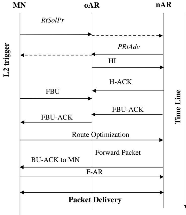
Figure 4.3: Message Exchange during Mobile IP Handover
