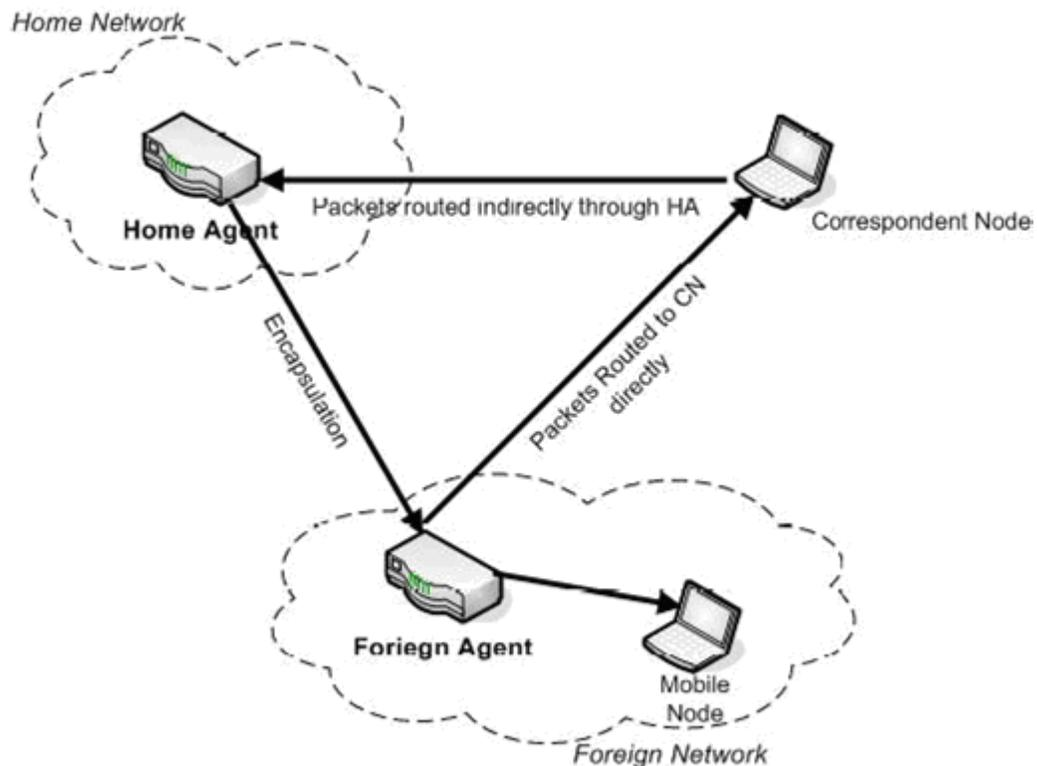
**Figure 2.2: Triangle Routing**
