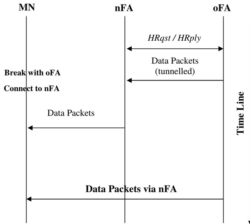
**Figure 2.6: Post-Registration Low Latency Handover Message Flow**
