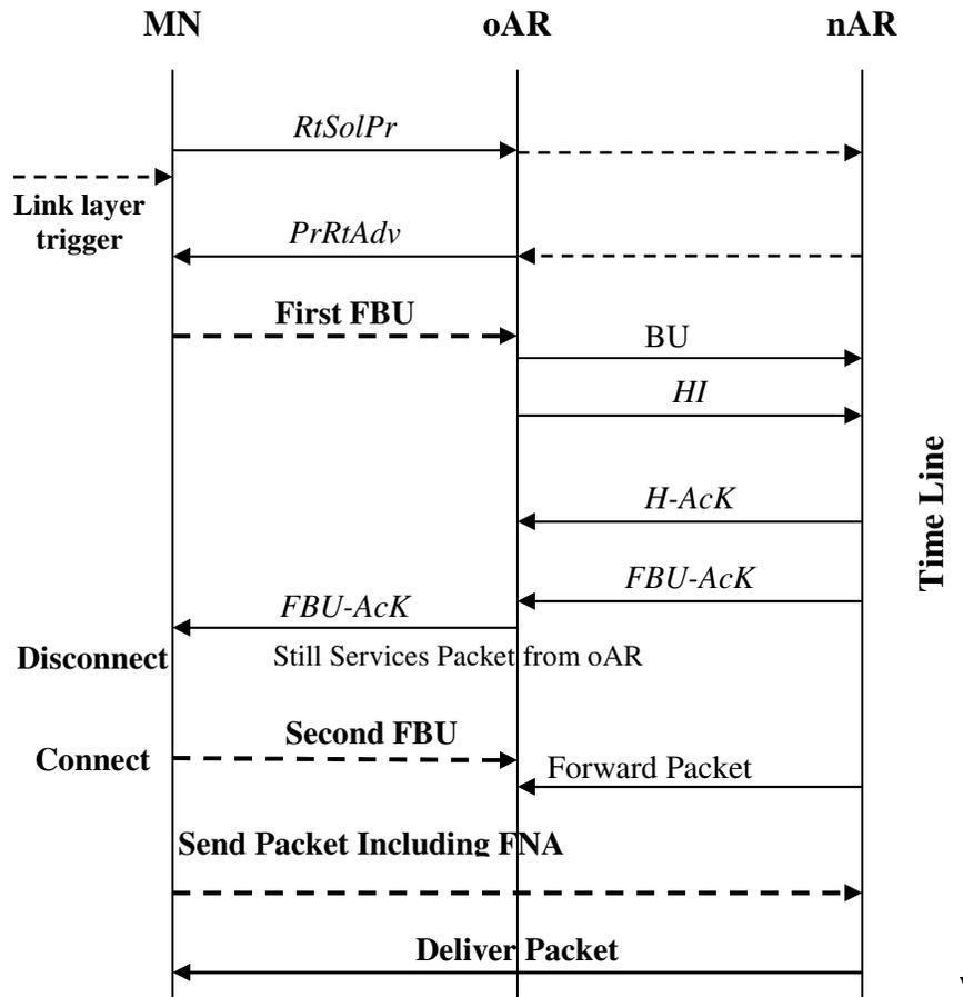
Figure 5.1: Fast Mobile IPv6 Handover Protocol Message Flow
