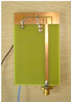
Fig. 3 Prototype antenna with DC bias circuit
