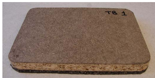
Figure 8.4: Shows multilayer product (base made from tyre shred residue waste, top chipboard)
