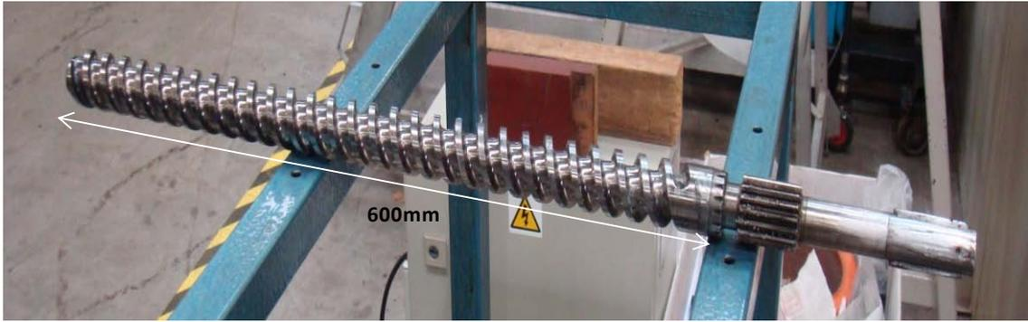
**Figure 7.11:** Screw used in the rubber extruder
