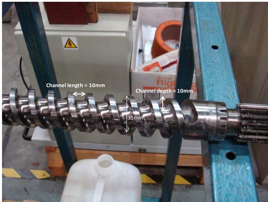
**Figure 7.12:** Screw channel and pitch
