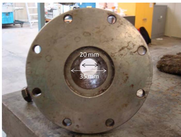
**Figure 7.10:** Die used at the end of the rubber extruder
