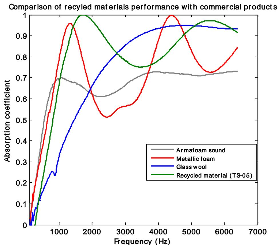
**Figure 7.7:** Comparison of recycled materials performance with commercial products (thickness = 25mm)
