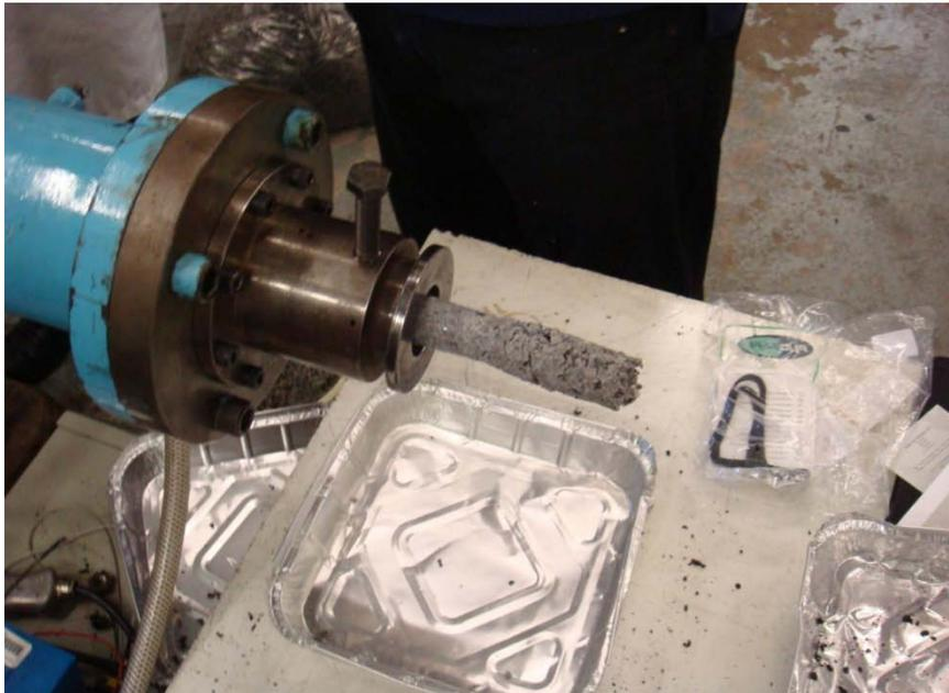
**Figure 7.9:** Picture of extrudate leaving the die
