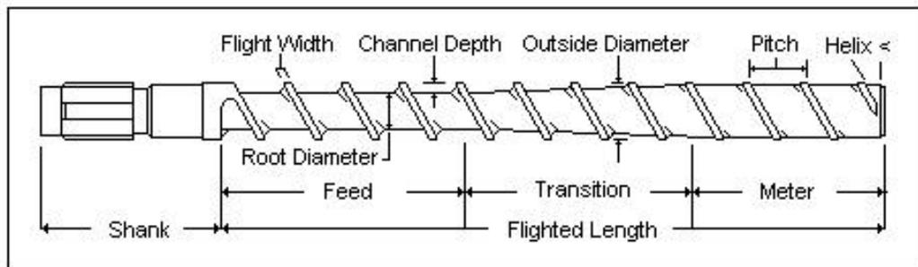
**Figure 7.13:** Schematic of standard screw used in hot extrusion
