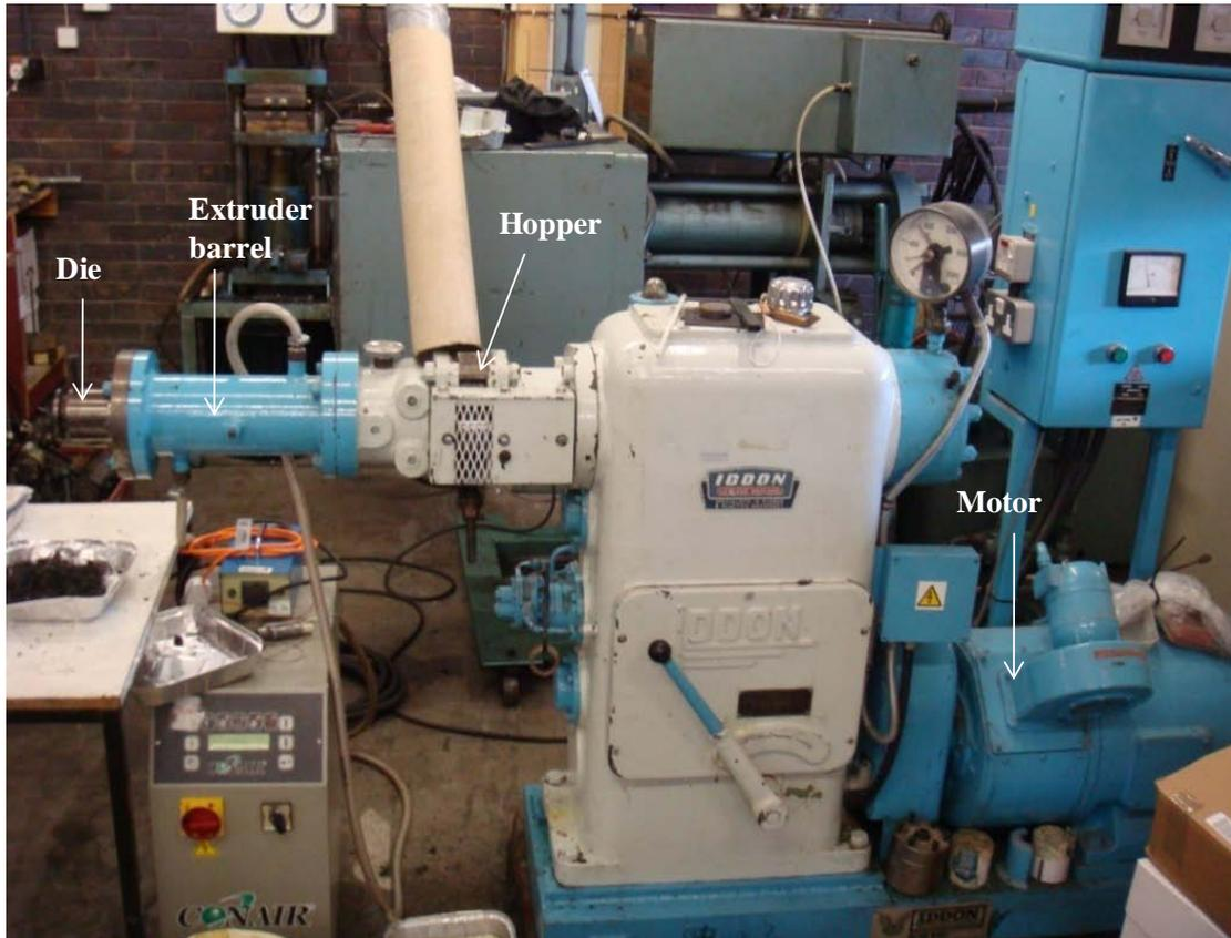
**Figure 7.8:** Rubber extruder at RAPRA
