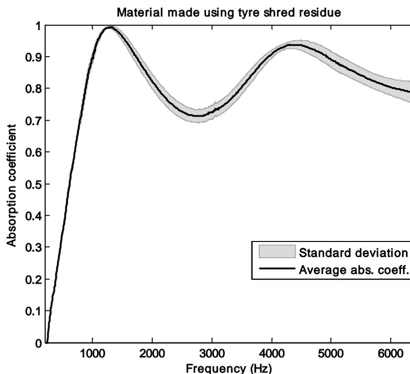
**Figure 7.6:** Material made using tyre shred residue TS-05 (thickness = 30mm)
