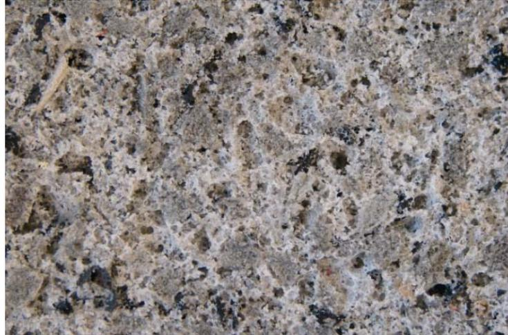
**Figure 7.5:** Picture of sample IM\_07 made using the formulation in Table 7.7
