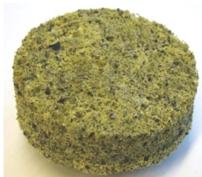
Figure 5.20: Picture of low density material made using tyre shred residue waste (YL01), formulation summary is given in appendix D
