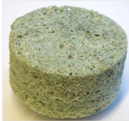
Figure 5.21: Picture of low density material made from carpet waste (ES10), formulation summary is given in appendix D
