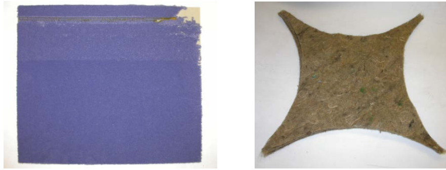
Figure 5.2: Defected PVC backed carpet tile (left) and trimming (right)
