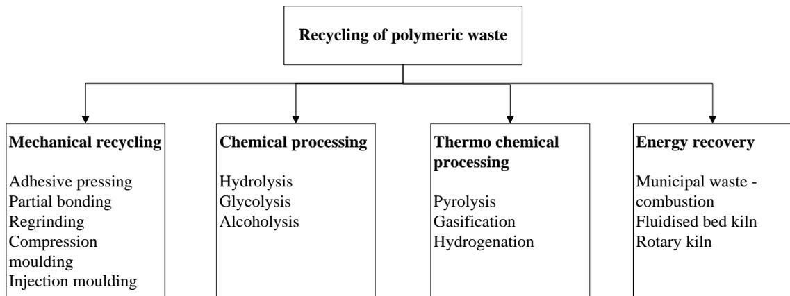
**Figure 2.8:** Overview of existing methods used to recycle polymeric waste
