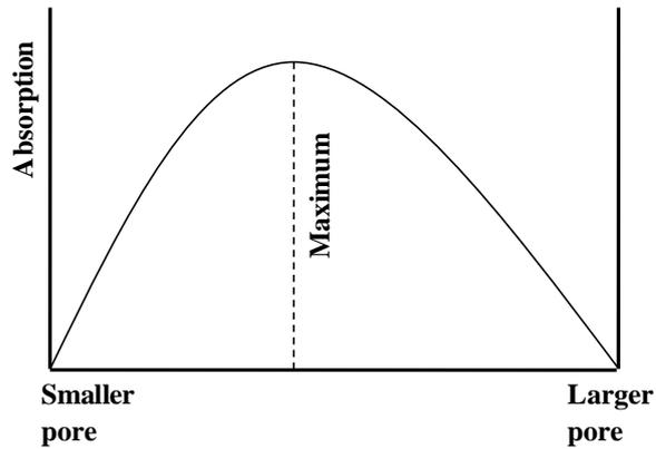
**Figure 2.1:** Absorption in a porous material
