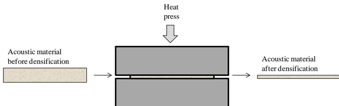
**Figure 2.7:** The Densification System
