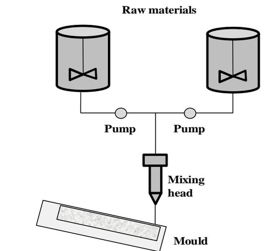
**Figure 2.4:** The Moulding System
