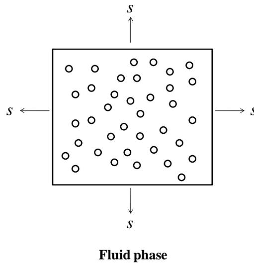
**Figure 2.13:** Stresses acting on the fluid phase
