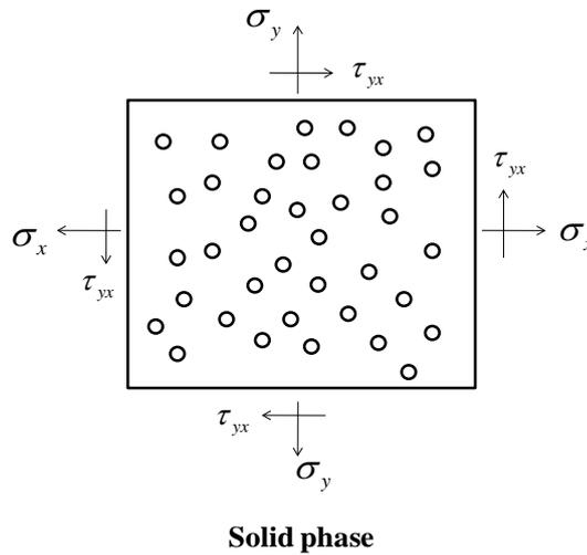
**Figure 2.12:** Stresses acting on the solid phase
