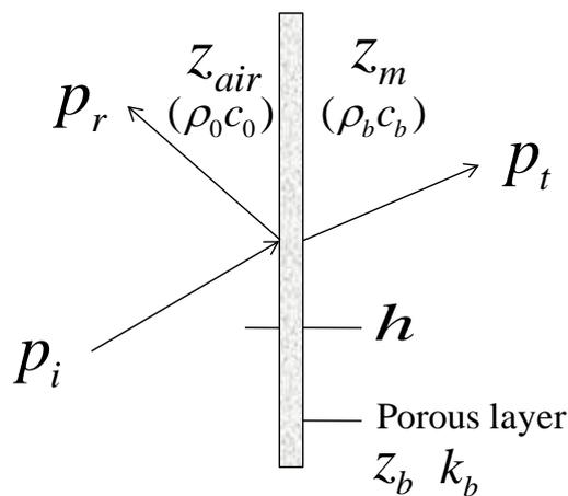
**Figure 2.11:** Sound wave reflection and transmission through a porous layer
