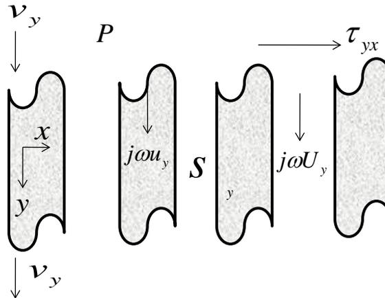
**Figure 2.14:** Boundary conditions for open surface
