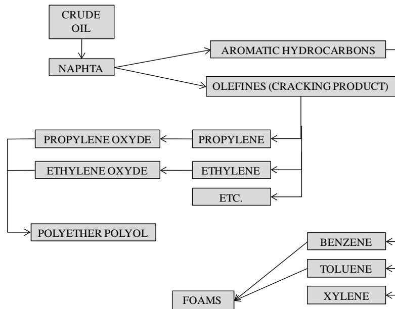
**Figure 2.2:** Flow diagram showing the origin of acoustic materials
