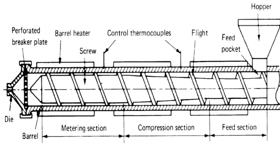
**Figure 2.15:** Schematic diagram of a standard extruder (Crawford, (1992))
