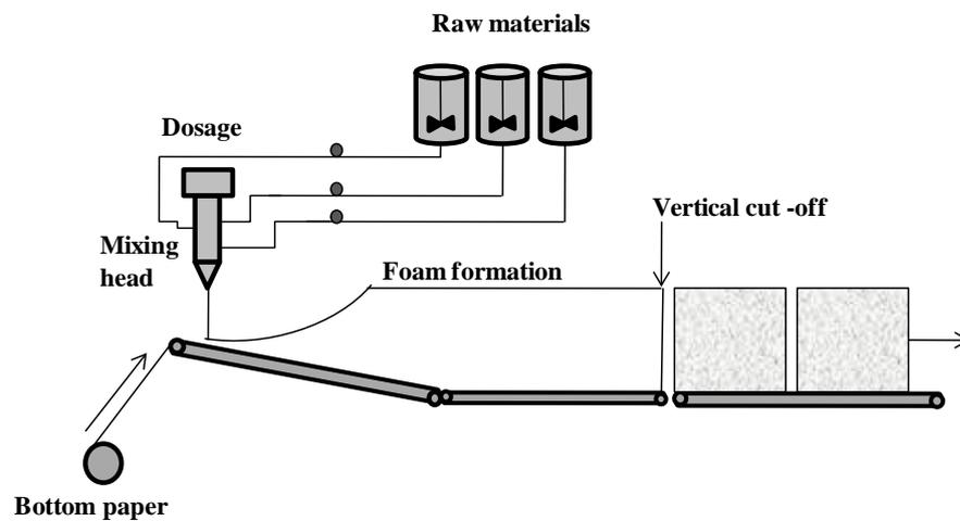
**Figure 2.3:** Inclined Conveyor System
