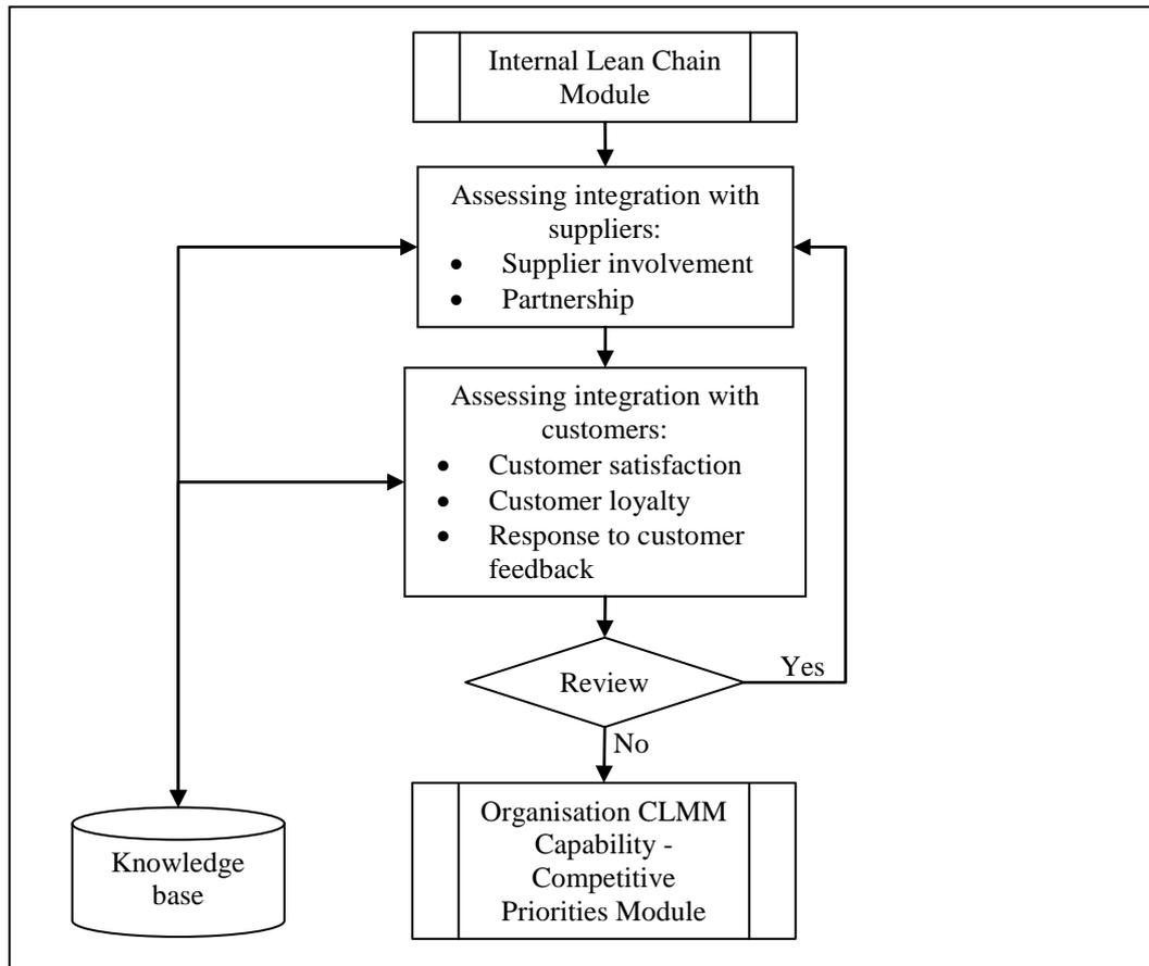
Figure 5.12: Flowchart of *External Lean Chain Module*
