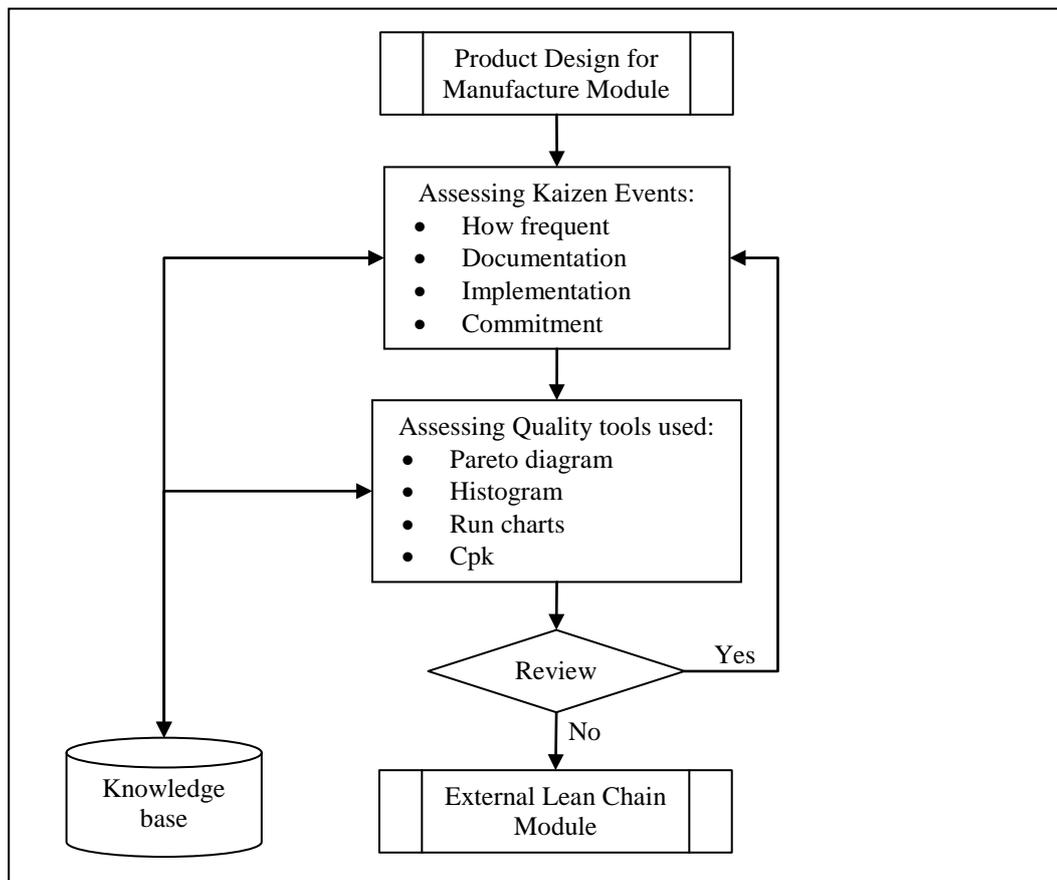
Figure 5.11: Flowchart of *Internal Lean Chain* Module
