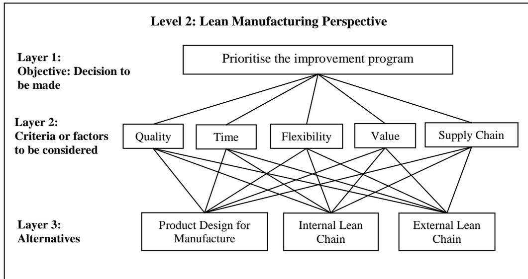
Figure 5.3: The AHP Structure for *Lean Manufacturing Perspective* of KBCLMM
