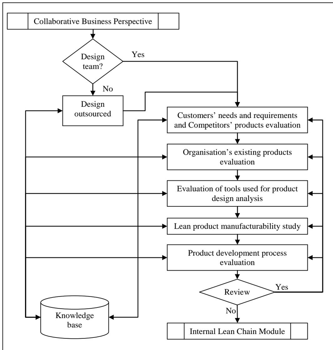
Figure 5.10: Flowchart of *Product Design for Manufacture* Module
