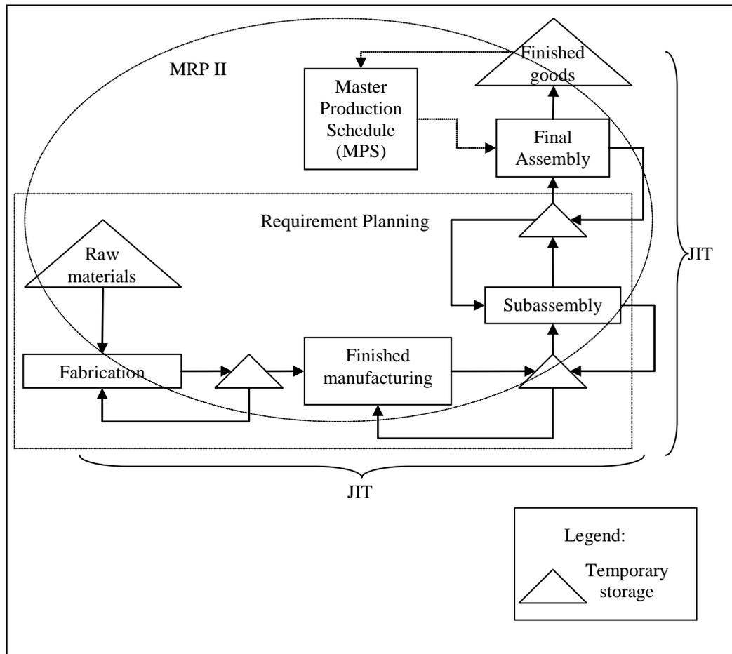
Figure 2.8: Production process control with integrated MRP II/JIT (adapted from Chase *et. al.* (2006))
