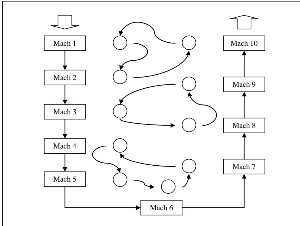
Figure 2.1: U-form Layout of a JIT Cell
