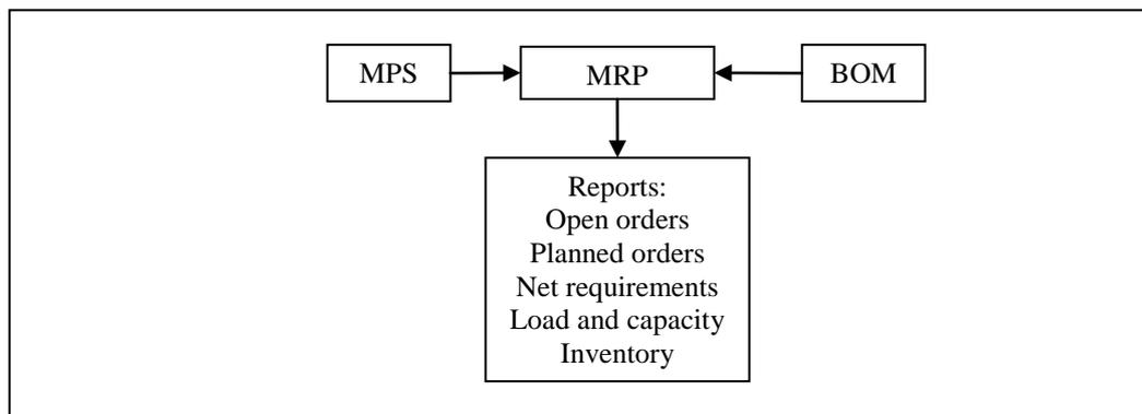
Figure 2.4: Structure of MRP (adapted from Buffa and Sarin 1987))
