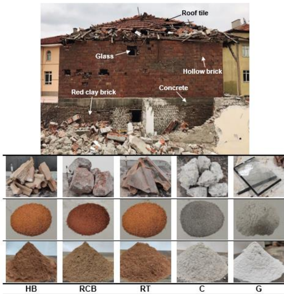
143 Fig. 1 A typical demolition site in Turkey and representative images of CDW-based materials 144 before crushing, after crushing and after grinding
