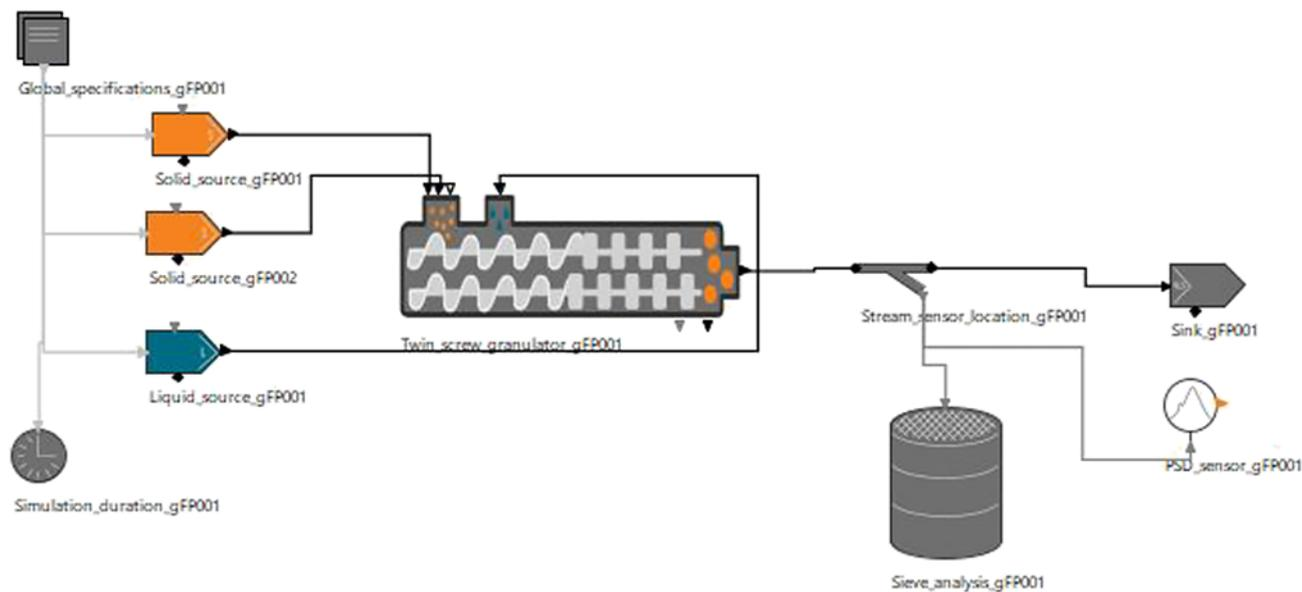
Figure 1. Flowsheet of the process made in gFP software.
