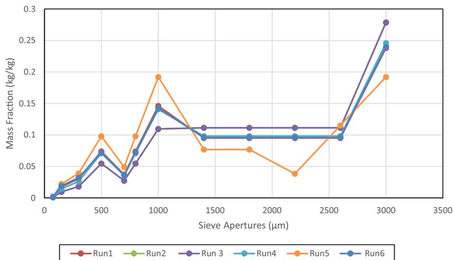
Figure 3. Granule size distribution for each screw configuration in the second set of simulations labeled (setup 2).
