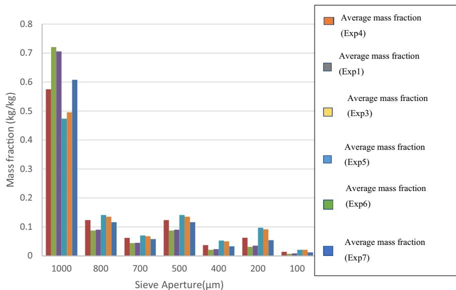
**Figure 2.** Chart of mass fraction for each screw configuration in the first set of simulations labeled "Exp".
