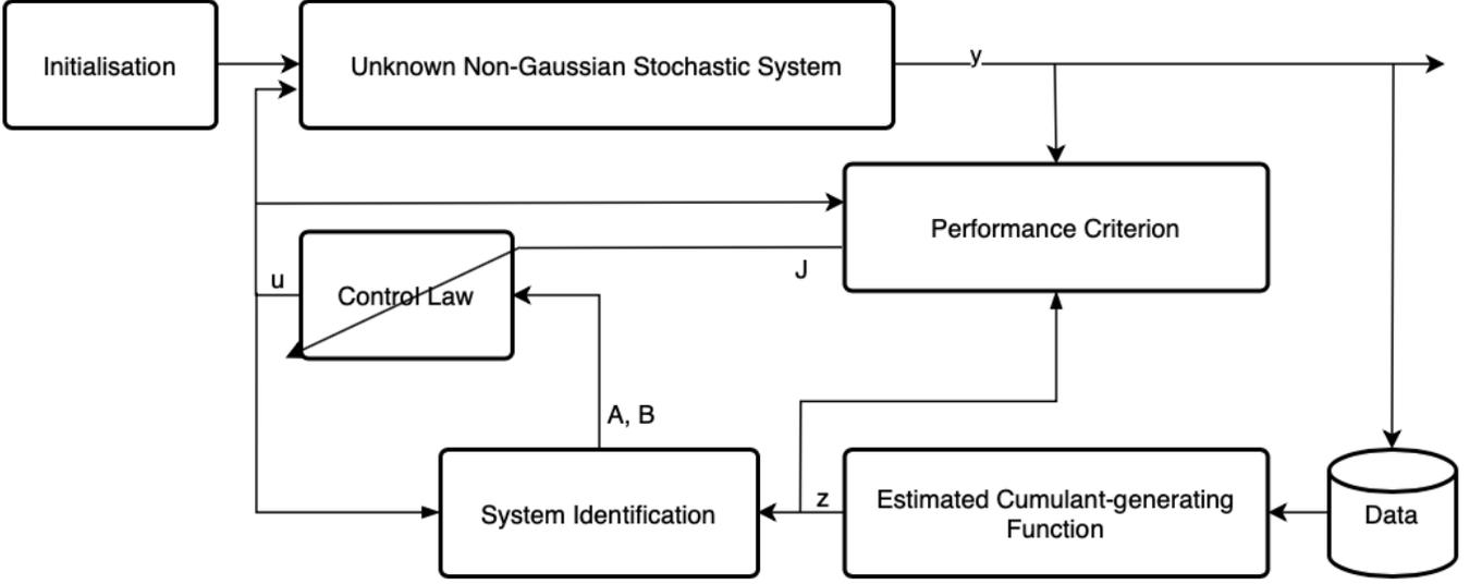
Fig. 2. Block diagram of the presented data-driven control algorithm.
