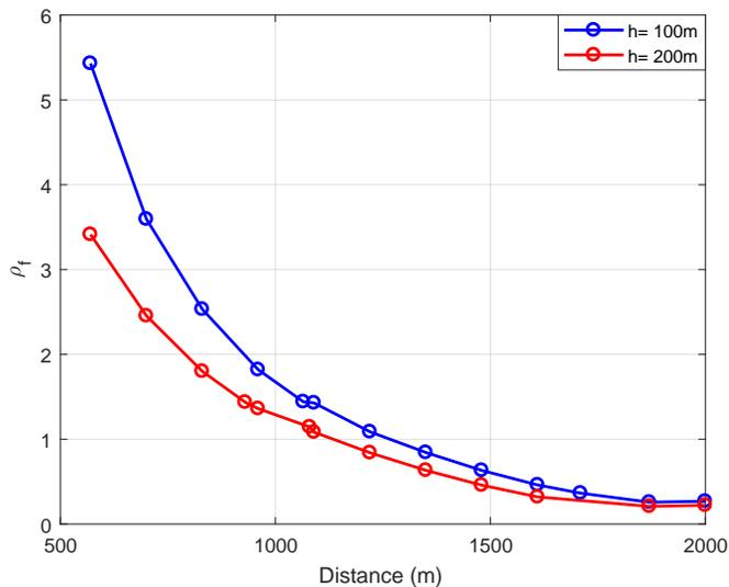
Fig. 6. Shrinkage rate index versus the aerial avoid-to-interference distance at various aerial altitudes
