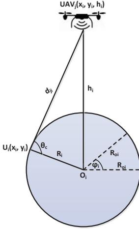
Fig. 1. A single UAV small cell coverage
