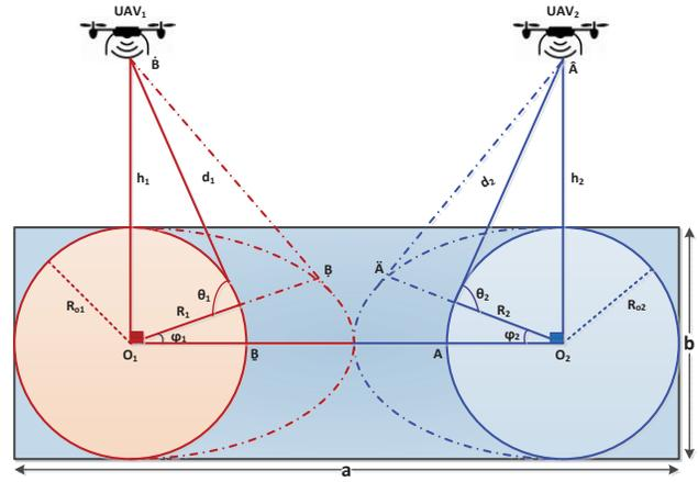
Fig. 3. Aerial coverage beam spots for multiple UAVs
