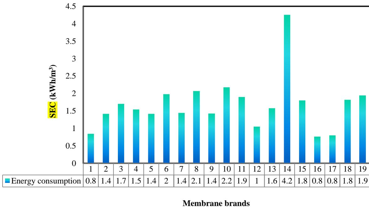
Fig. 6. Impact of membrane brands on the SEC of RO system
