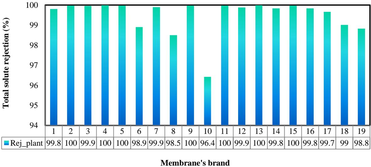
13 **Fig. 2.** Impact of membrane brands on total solute rejection of RO system
