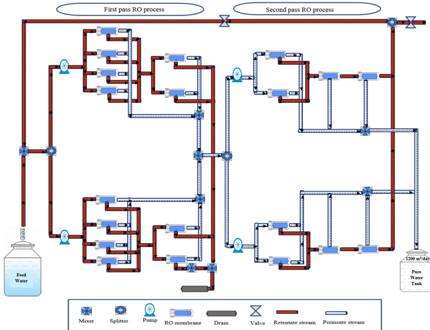
Fig. 1. Layout of BWRO desalination plant of APC (Adapted from Al-Obaidi et al. [31])
