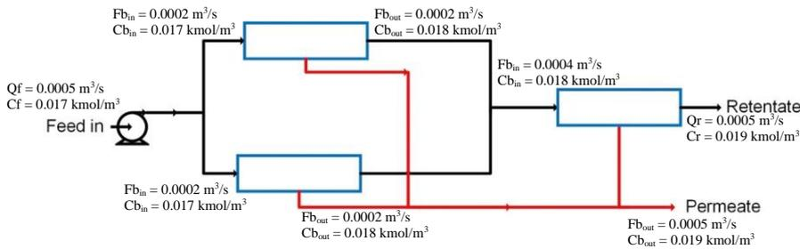
Fig. 5. RO tapered 2-1 configuration
