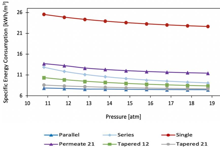
Fig. 10. Effect of pressure on SEC for five multistage configurations and single membrane
