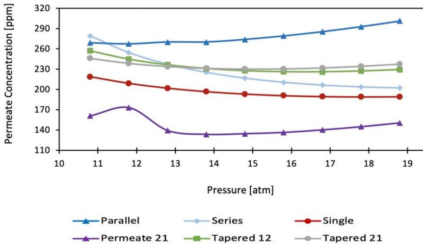
Fig. 8. The effect of pressure on permeate concentration for five multistage configurations and single membrane
