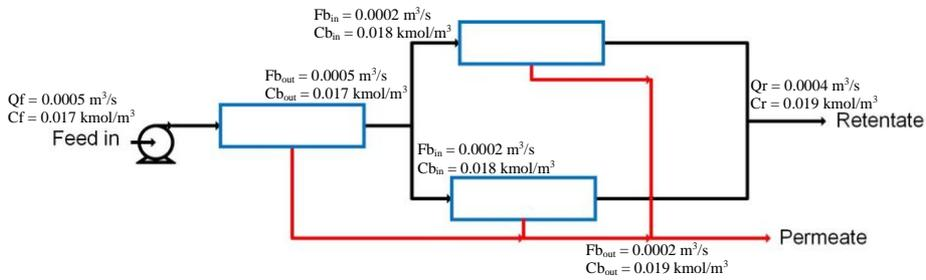
Fig. 4. RO tapered 1-2 configuration
