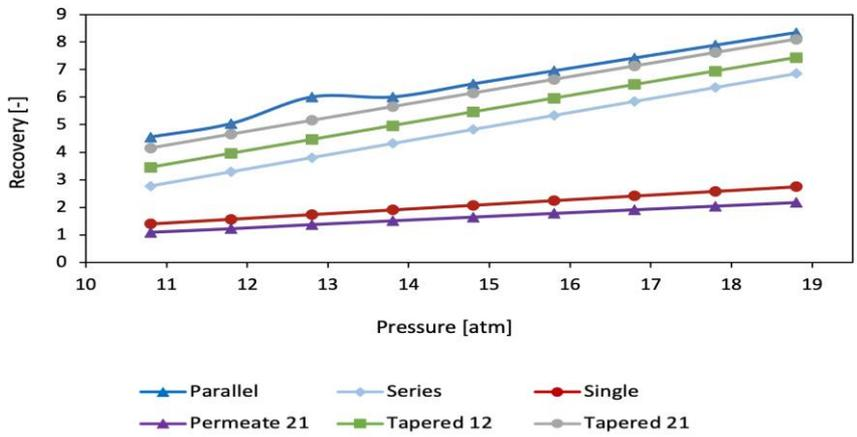
7 **Fig. 9.** Effect of pressure on water recovery (yield) for five multistage configurations and single membrane
