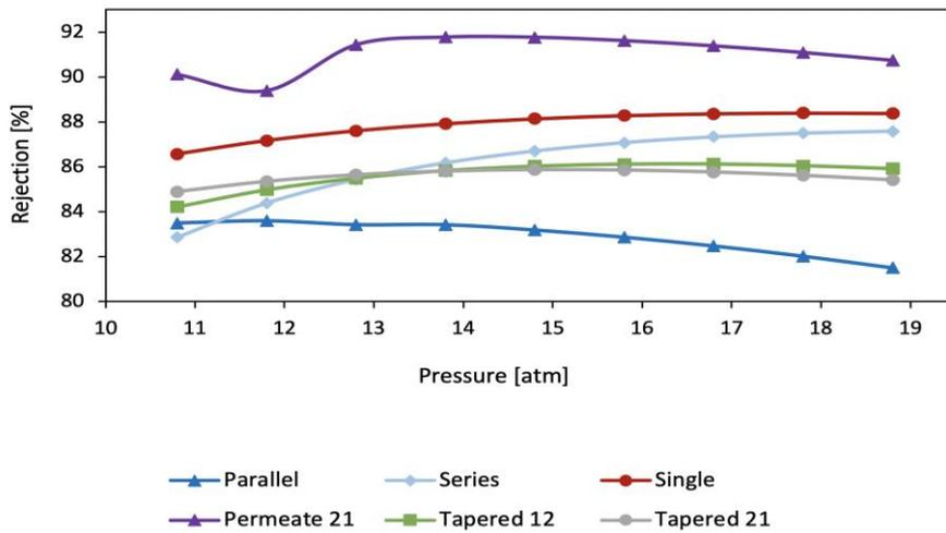
Fig. 7. The effect of applied pressure on phenol rejection for five multistage configurations and single membrane
