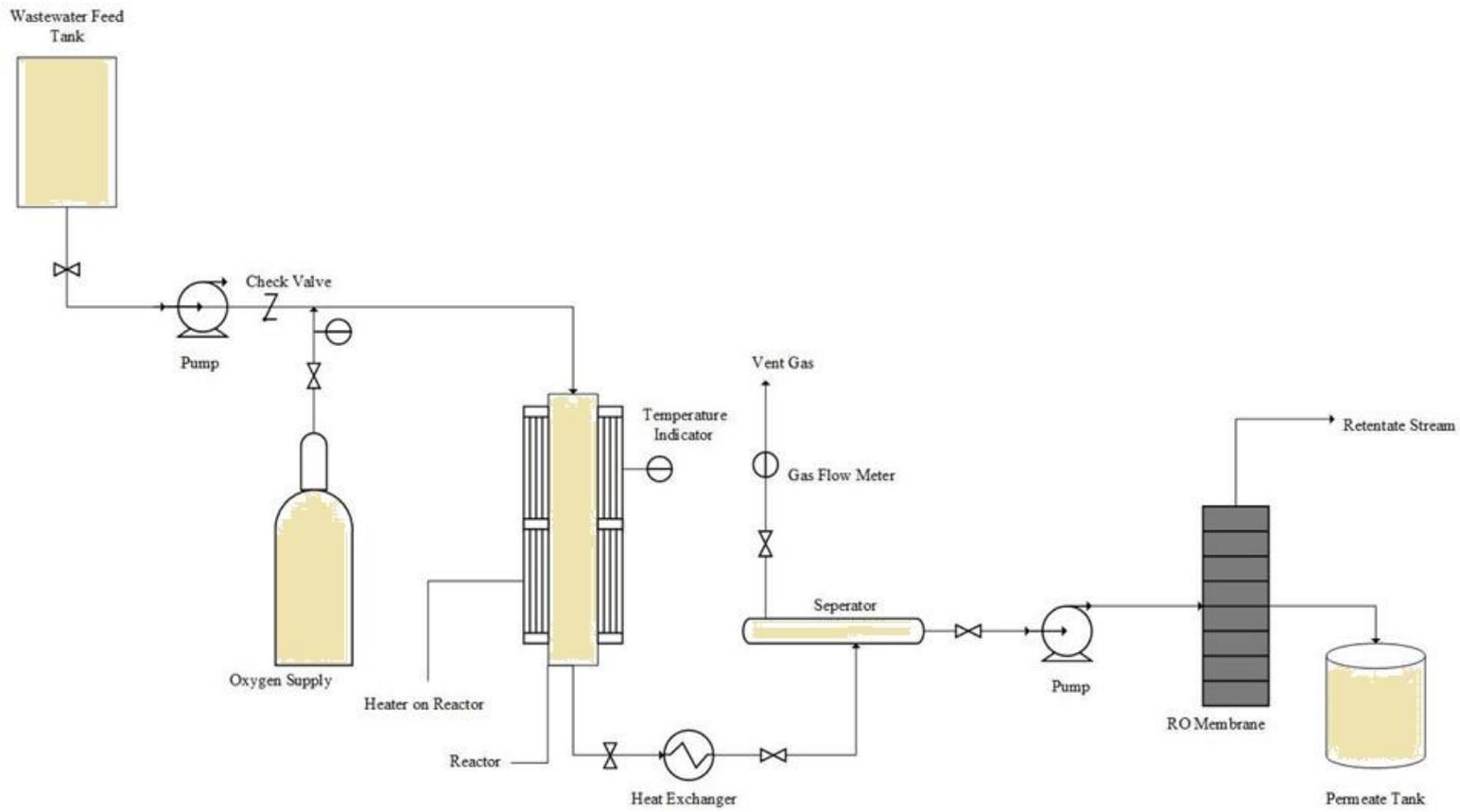
Fig. 1. Process flow diagram of the TBR-RO hybrid system (Adapted from Al-Obaidi et al., 2018a)
