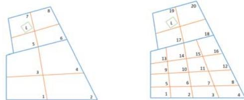
Fig. 5. Domain discretisation (left: First refinement, right: second refinement only in the lower trapezium).
